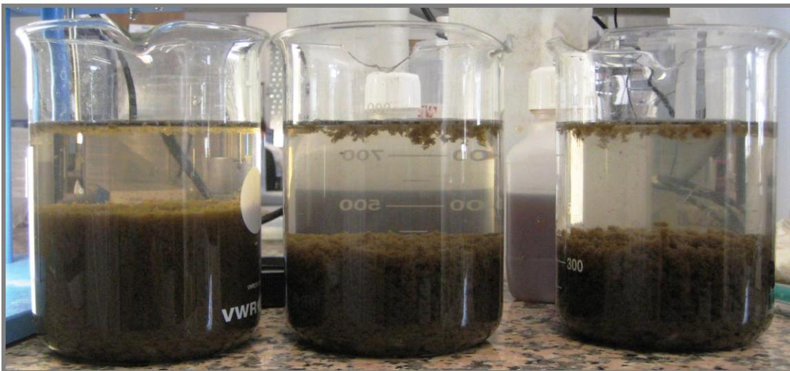
**Figure 1.** From left to right, Test 1 (ferric chloride), Test 2 (ADNATUR K70) and Test 3 (ADNATUR K20).
